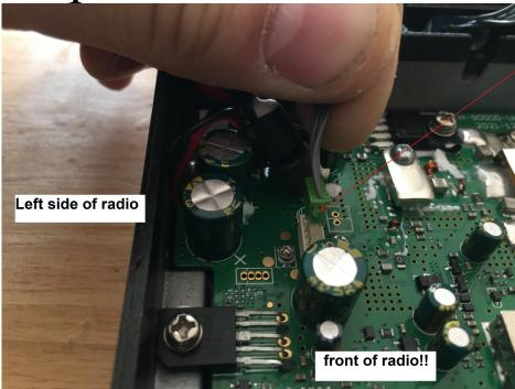
NOTE: the TAB on the plug!! the tab needs to be facing the way you see it in the picture!!
